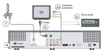
Figure 52: Connecting a standard TV (480i) and stereo audio
